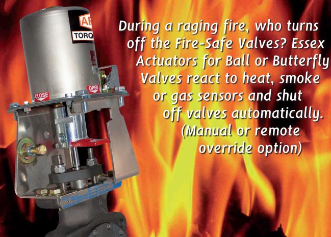
A thermal heat activated or electrothermal ball/butterfly valve fitted with an enclosed compact spring pack, mechanical actuator that can sense heat or smoke as well as a gas leak and shut off (or open) automatically. Thermal shut-off at your choice of temperatures from 135° to 500°F (57° to 260°C) with UL listed enclosed thermal link is rugged, reliable, compact, economical and intrinsically safe. FM approval available.
