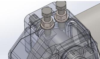
Please note to tighten the bolt nut after adjusting the appropriate on/off position.
