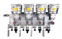
The ARCS is a redundant solenoid valve piloting system for emergency shutdown valves. Available in various redundant configurations—1002, 2002 and 2003—the system achieves a higher level of process safety and reliability.
