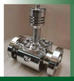
Cryogenic TOP ENTRY ball valves, floating ball and trunnion mounted execution. Available from ½" to 36" class 150 to 2500. Forged stainless steel material up to 3" and European castings for bigger sizes. Easy in-line maintenance
