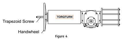
After manual operation, screw out the trapezoid screw until the spring is disengaged toward the actuator to return to auto-operation, check to ensure the spring can open fully and the spring is totally disengaged from the jackscrew. Avoid fully screwing out integral the trapezoid screw, as the screws also act as a position stop to ensure the valve is correctly returned to the full open or close position.
