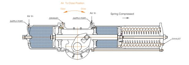
\* Open/Closed is relative to mounting on valve and assumes valve has actuator mounted to "fail closed". Valve/Actuator can also be mounted "fail open".
