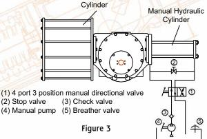
mounted on the pneumatic actuator, close ball valve (2) by operating the hand pilot valve to control the hydraulic cylinder's oil supply/exhaust, and operate the hand pump to energise opening or closing the valve manually. To return to automatic operation, set the handle of the 4 port 3 position manual direction valve (1) to the middle position and open ball valve (2), Manual over-ride is then disengaged.
