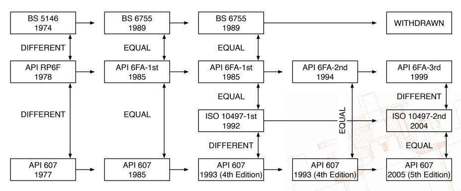
API 607 4th Edition & ISO 10497 - within 10 minutes after extinguishing the flames valve temperature must be below 100°C cooling with water spray. Rest of standards unforced cooling down.
