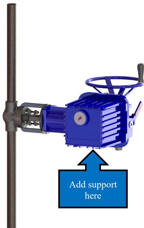
Figure 15 - Supporting a Motor-Operated Valve
