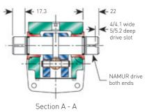
MODELS 023 THROUGH 100 - TOP AND BOTTOM OF HOUSING (SYMMETRICAL) ISO 5211-F12
