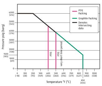
\*Temperature also limited by seat and seals. Special bonnet may be required for high temperature service above 300°C.
