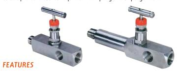
316 S.S. construction for corrosion resistance. Non rotating vee or ball tip. Extended body for insulation clearance. Scheduled 160 or heavier pipe valve inlet for strength. Optional graphoil packing available for high temperatures. Ball\*/vee tip design forms a bearing joint with the stem which eliminates rotation between ball/vee tip and seat at closure. This prevents scoring and galling up the valve seat and ensures long life in repetitive shut off service.
