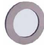
Mechanically pre-stressed fused metal ring with encapsulated borosilicate glass insert option up to 600 class.
