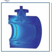
Starline uses the FEA for designing its compact ball valves. Finite Element Analysis (FEA) is a very important step of the development stage and ensures the best possible performance requirements. Valves operational problems, pressure/temperature related deformations and flow-related forces within a valve can be evaluated.
