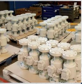
All the **Starline** API 6A ball valves are identified on proper name plate and on valve body as required by API 6A, MSS-SP 25, ASME B16.34.
