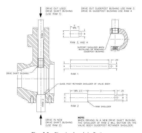
Figure 5. Ram Dimensions for replacing Bearings
