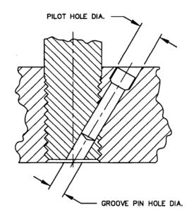
Figure 2: Groove Pin Pilot Holes
