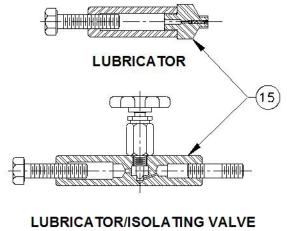
Figure 3: Lubricator and Lubricator/Isolating Valve
