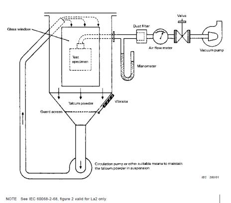
Figure 2 – Test device to verify protection against dust (dust chamber)
